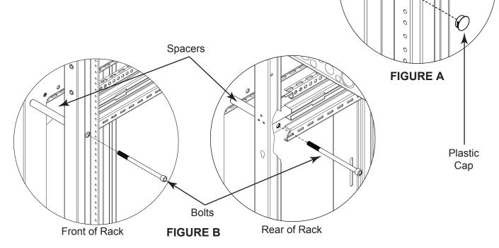
3) Install cable chase bottoms onto spacers located at the front and rear of joined racks. Install front and rear tops once bottoms are in place. (FIGURE C)
