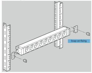
Vertical mounting possible by turning the fixing brackets round and positioning them on the rear of the unit.
