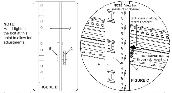
4. Repeat the previous steps to match the hardware amounts (hex head bolts and rackrail nuts) to the amount of rackrail brackets in your enclosure.
