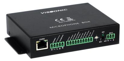
The VIS-AIB microphone interface box is designed to support VISSONIC conference microphone remotely installed under the table or armrest solution. With the phoenix connectors on both sides of the box, it can connect Dynamic mic/Boundary Condenser mic input, buttons and speakers on plate to control the conference unit etc. By the RJ45 port it can easily connect into existing VISSONIC conference microphone family to integrated into one part seamlessly.
