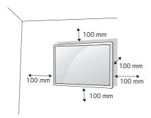
To install your monitor on a wall, attach a wall mounting bracket (optional part) to the back of the monitor. Make sure that the wall mounting bracket is securely fixed to the monitor and to the wall.
