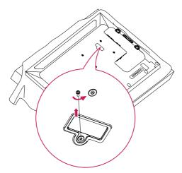
2 Align the WP401/WP402 along the four screw holes on the rear of the set and attach it to the rear of the set using the four screws provided.
