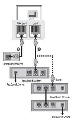
Connect the LAN port of the Modem or Router to the LAN port on the TV.
