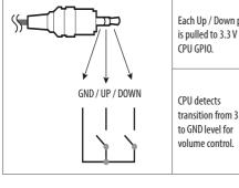
Each Up / Down pin is pulled to 3.3 V with
