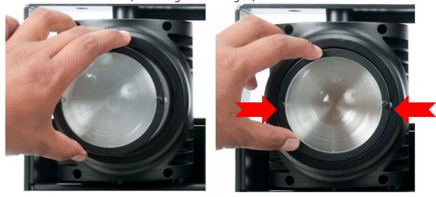
**3.** While applying gentle pressure against the lens, slowly turn the lens counterclockwise a ¼ turn, until both small black raised plastic tabs are positioned vertical at 12 and 6 o'clock.
