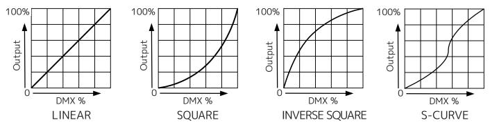
The S-Curve Dimmer Curve is ideal for controlling a blinder-type fixture, as it features a smooth bottom and has no harsh reduction in lighting intensity when fading down from 100% output. When operating in a DTW-enabled setting with manual fader control, the S-Curve will provide the most natural feel.
