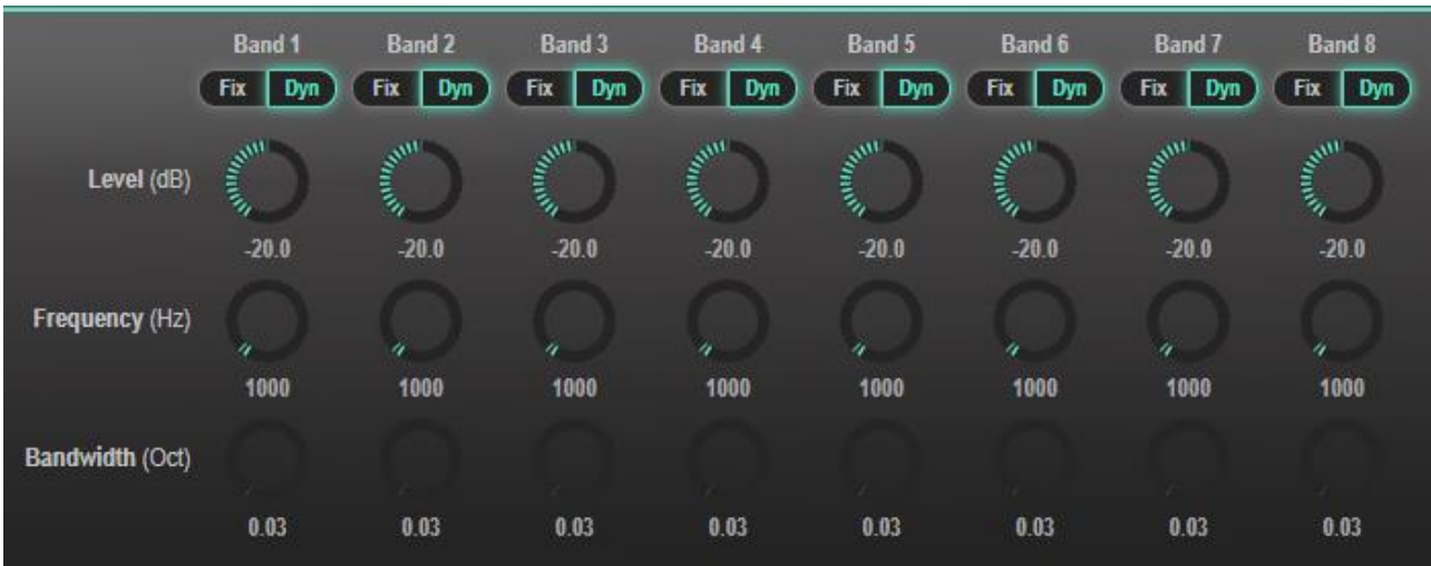
Figure 31: AFS Module – Selecting Input Fixed or Dynamic AFS Band Values
