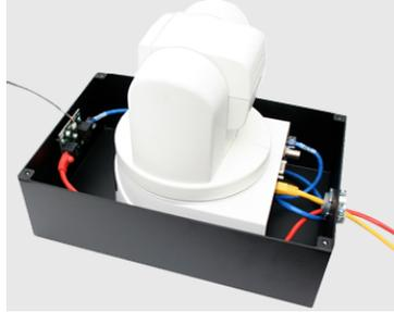
Other HD-series cameras have shorter bases. If you are installing an HD-20, HD-20SE, HD-22, HD-30, or HD-USB camera, use the long  $\frac{1}{4}$ -20 screws with the spacer block to attach the camera to the enclosure.
