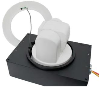
3. Pass the excess length of cable (if used) into the enclosure as you raise the trim ring into place.
