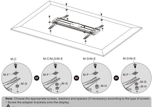
Tighten all screws but do not over tighten.
