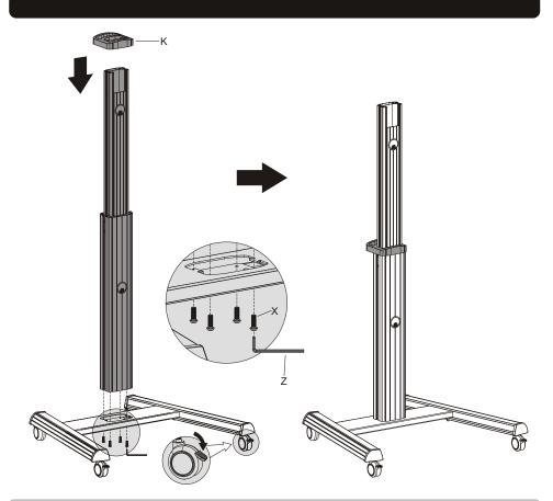
Attach the column to the base using the screws. Tighten all screws using an allen key.
