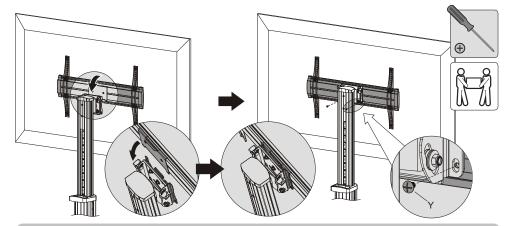
· Hook the universal plate onto the support plate.
