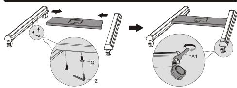
Insert the right leg into the base. Align the holes in the right leg to the holes in the base. Secure with the screws. Repeat this step for the left leg.
