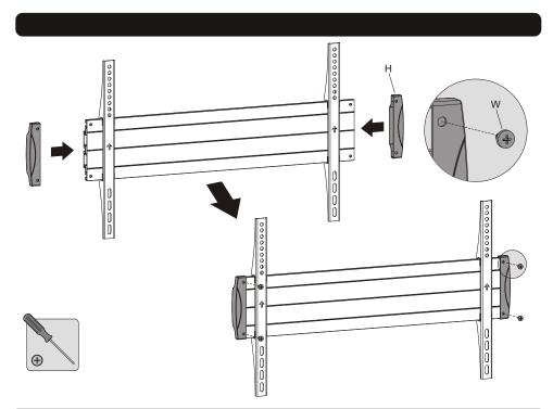
Attach the two plastic covers to both ends of the plate using the appropriate screws. Tighten all screw using a suitable screwdriver.
